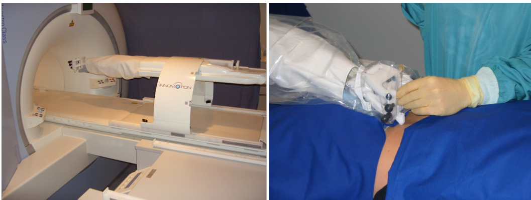
Figure 2.8: Innomotion™ robot-assisted system and Innomotion™ AMO biopsy needle guide for percutaneous intervention under CT/MRI. Image Source: INNOMEDIC
