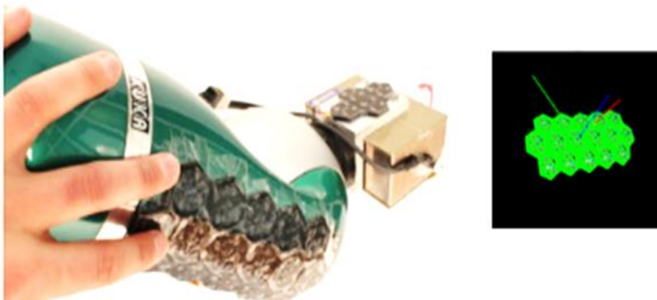
Figure 2.3.7 3D Reconstruction of a KUKA LWR arm [99]. The sensors are covered on the arm. The orientation of each sensor patch is transmitted to the micro-controller unit.
