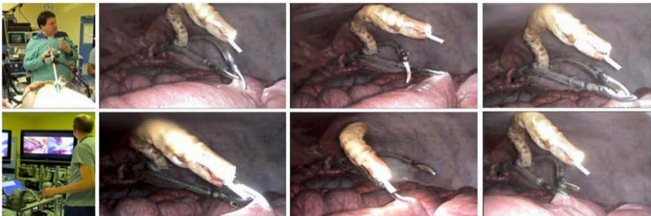
Fig. 8 One surgen operating the instrumetns and another surgen operating the arms. The robot was deployed trans-vaginally, performing small bowel inspection.
