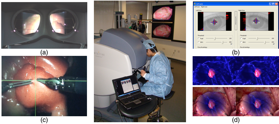
Fig. 1. The experimental setup for the gaze-contingent perceptual docking studies (centre). A binocular eye tracker (a, b, c) is integrated in the daVinci surgical console and a 6-DOF haptic device is used for the experiments. d) Eye tracking is also used for gaze-contingent augmented reality [16].
