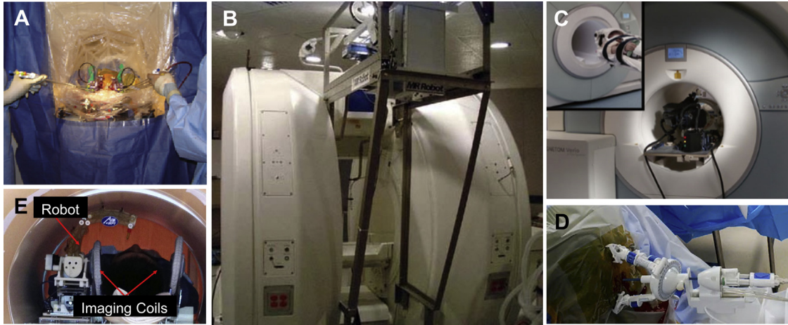
FIGURE 34.2 Significant MRI-guided stereotactic neurosurgical systems. (A) ClearPoint system by MRI Interventions, Inc., United States. Two frames (SmartFrame) are mounted to the skull bilaterally and manually aligned to the predefined trajectories [18,19]; (B) MRI-compatible surgical assist robot by AIST-MITI, Japan and BWH, Harvard Medical School, United States [20]; (C) NeuroArm/SYMBIS by Deerfield Imaging, United States [21]; (D) NeuroBlade system by Monteris Medical, Inc., United States [22]; (E) a MRI-guided stereotactic robot for deep brain stimulation, developed by Worcester Polytechnic Institute, United States [23]. MRI , Magnetic resonance imaging.
