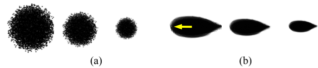
Fig.4. (a) Spray paint templates under different painting depth descending from left to right; (b) another brush templates in water drop shape with front direction defined which is shown by the arrow
