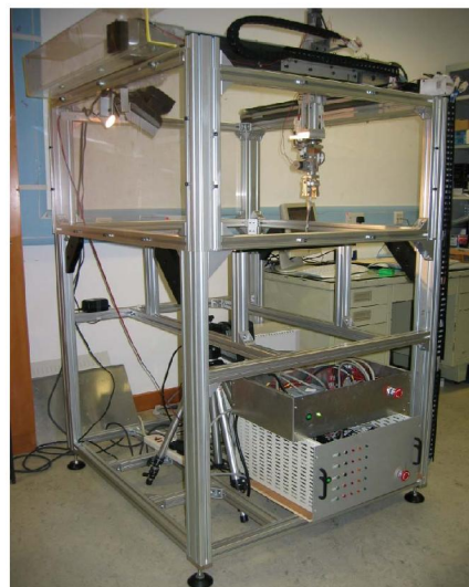
Fig.2. Hardware Design of the Drawing Robot
