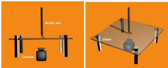
Fig.3. Conceptual idea and hardware for footprint acquisition
