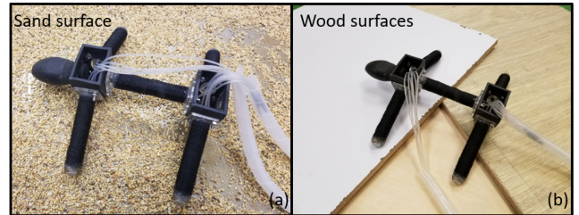
FIG. 5. (a) Quad pedal walking on sand surfaces; (b) on wood surface
