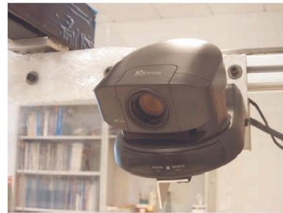
Figure 3. Camera looking down at drawing area for monitoring and visual-based capabilities
