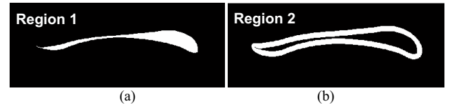
Fig.12. The sample stroke is divided into two regions in white: (a) inner region, (b) outer region, those are inside the stroke
